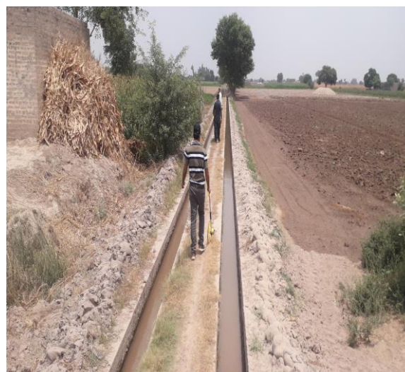
Measuring Lining Length of W/C with Measuring Wheel
